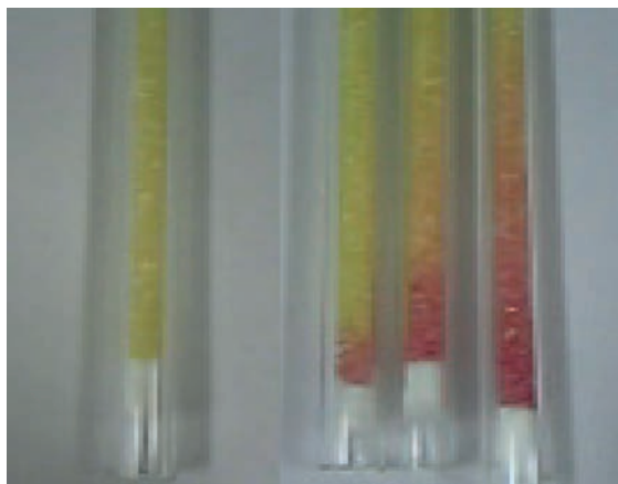
Figure 3. Color changes of the detector tube after pumping a 100-mL indole-mixed air. Concentration of indole vapor in air was 0.0 (as a blank), 2, 6, and 10 ppm, respectively, from the left.
